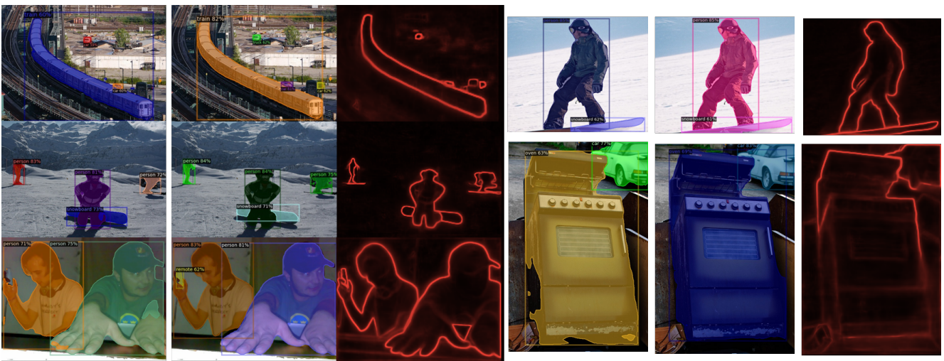
Figure 9. Qualitative Comparisons on the Boundary Area. (left) the results from BlendMask [6] (middle) the results from ours (right) the corresponding learned image boundary basis.
